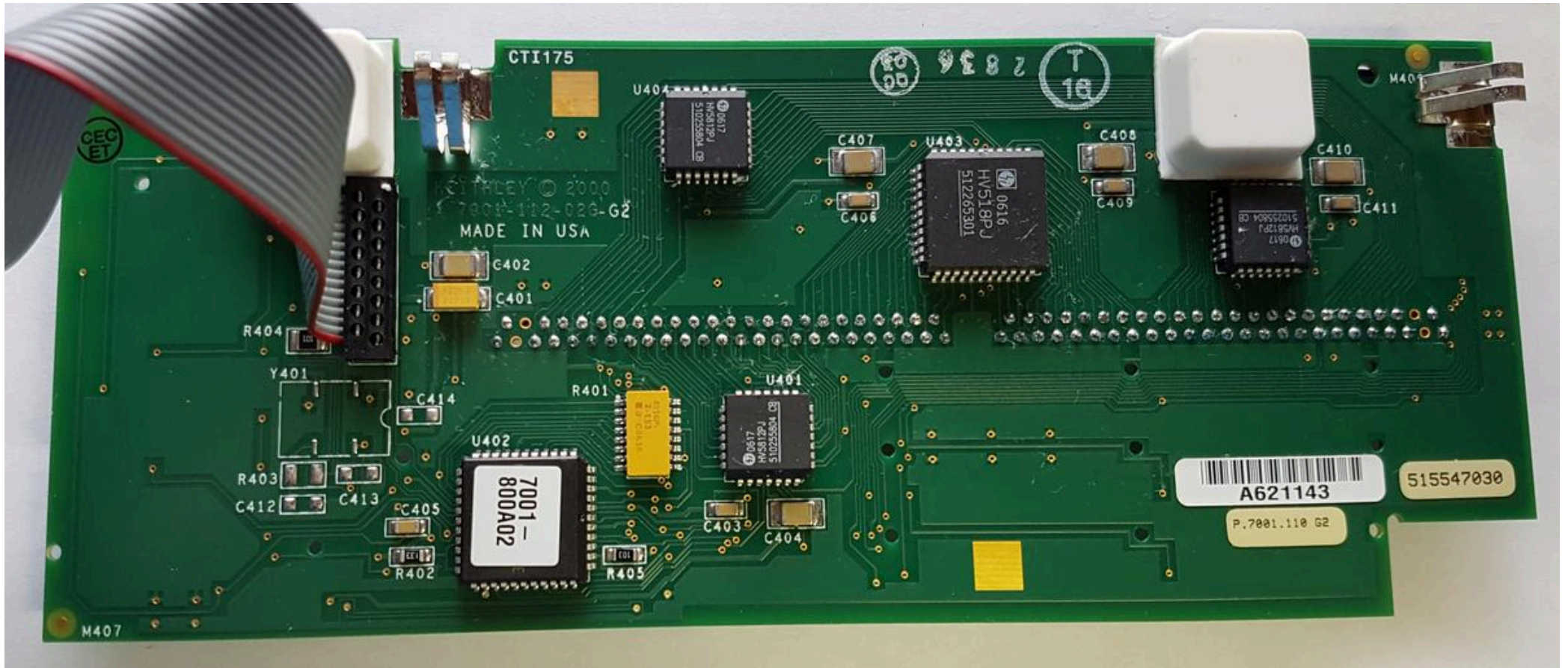
Itron DD-51, Older xDevs.com's Keithley 2002 (PCBA manufactured around 1995 week 2)
